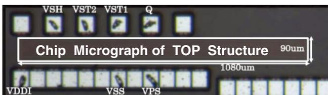
**Fig. 8.** (Color online) Chip micrograph fabricated in a 65 nm CMOS.
