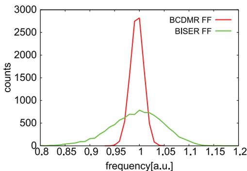
**Fig. 7** Variations of BCDMR and BISER to fluctuate  $V_{th}$  of transistors in C-elements and weak keepers.
