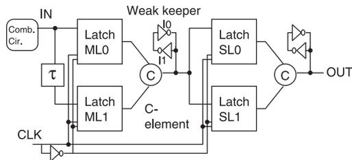
Fig. 1 BISER FF and inverting Muller C-element.
