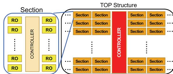
**Fig. 8** Conventional matrix-array-based (MAB) test structure.
