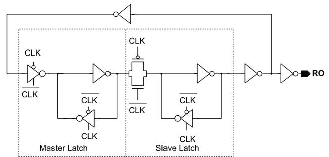
Fig. 3 Ring oscillator implemented with master and slave latches. Both latches are negative to utilize CLK as the enable signal for oscillation.
