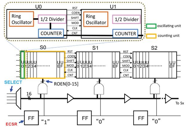
**Fig. 10** Block diagram of the shift-register-based test structure.
