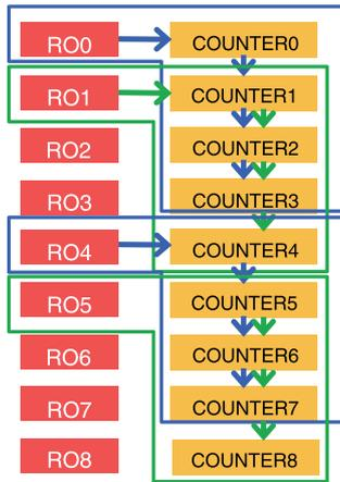
**Fig. 9** Conceptual block diagram of the shift-register-based test structure. Oscillating waveform of RO1 is captured by COUNTER[3-0].
