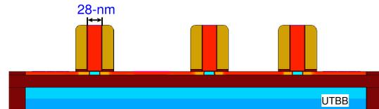
(b) The cross-section of 3D NMOS device model in the 28-nm UTBB structure.
