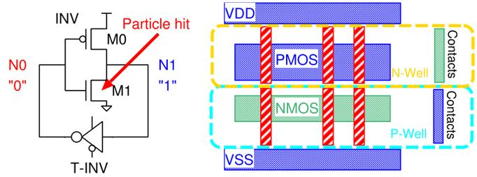
Fig. 4. Circuit and Layout structure of a conventional latch.
