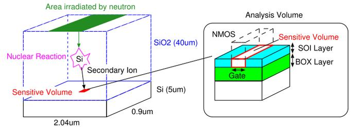
Fig. 3. Configuration of test device structure used in PHITS simulations. The SOI layers under G is regarded as the sensitive volume of the latch according to the TCAD simulation.
