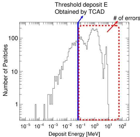
Fig. 2. PHITS calculation of the deposited energy. Each particle, with deposited energy exceeding the threshold energy, is counted as one SEU.
