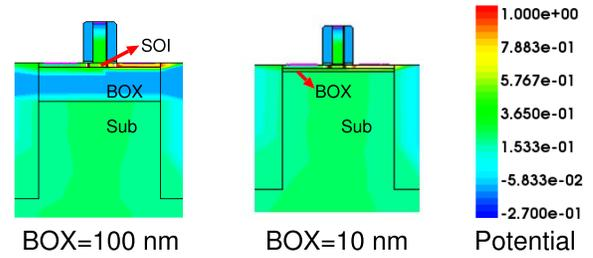
Fig. 11. The potential 10ns later a particle hits. The potential of the 10 nm BOX layer is higher than that of 100 nm thick BOX layer.
