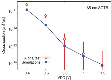
(a) The cross-section in SOTB structure according to the alpha irradiation experiments and simulations.
