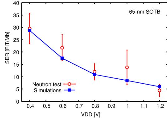
(a) The SERs of SOTB structure according to the neutron irradiation experiments and simulations.
