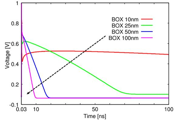
(b) The potentials of SOI layer depending on the thicknesses of BOX layer. It becomes easier to turn on the parasitic bipolar transistor when the thickness of BOX layer is much thinner.
