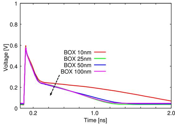
(b) The potentials of SOI layer depending for varying BOX layer thickness. It becomes easier to turn on the parasitic bipolar transistor when the BOX layer is much thinner.
