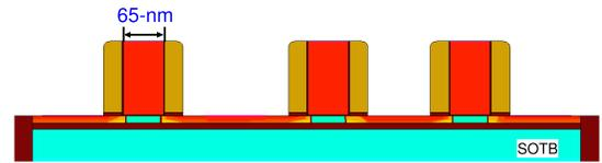
(a) The cross-section of 3D NMOS device model in the 65-nm SOTB structure.
