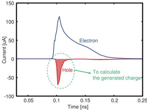
Fig. 6. Current waveforms by a particle hit. Blue current pulse is generated by electron collection, while the red is generated by hole collection. The generated charge collected by drift and diffusion is used to calculate  $Q_{th}$ .
