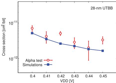
(b) The cross-section in UTBB structure according to the alpha irradiation experiments and simulations.
