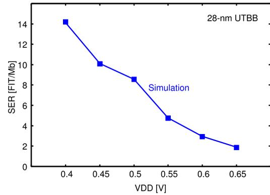
(b) The SERs of UTBB structure according to the simulations.
