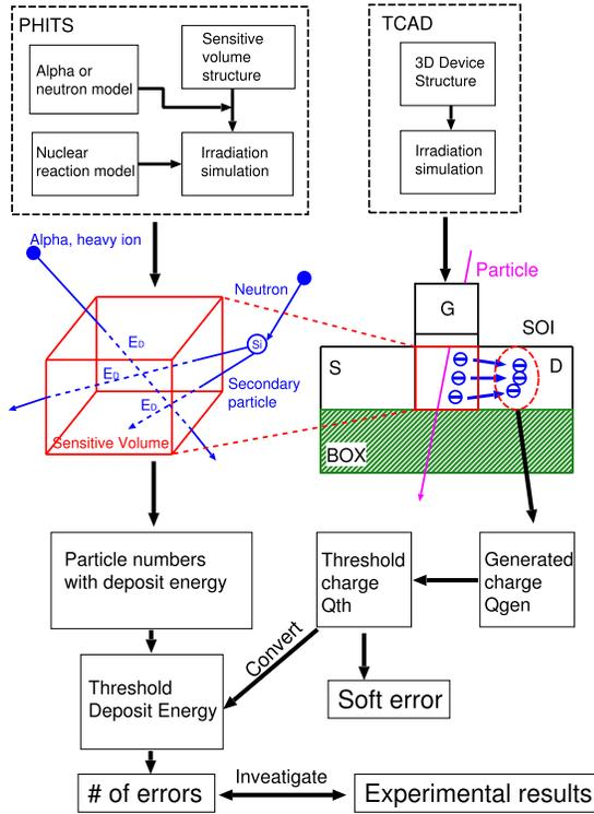
Fig. 1. Flow chart of the Monte Carlo PHITS and TCAD simulation system.
