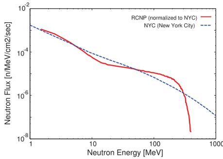
Fig. 7. Energy spectrum of spallation neutron beam.
