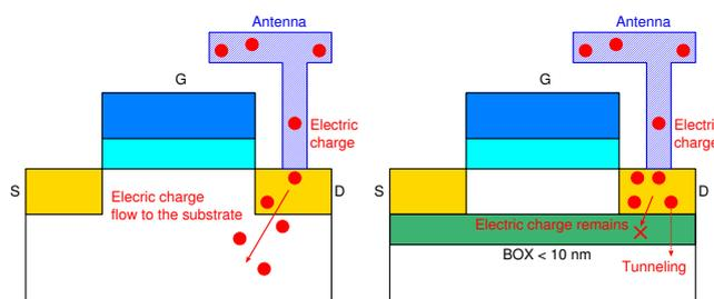
Fig. 3. Relieving PID in the Drain of Bulk
