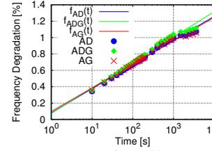
Fig. 13. BTI of AR500 in the SOTB Process
