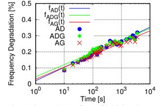
Fig. 12. BTI of AR6250 in the Bulk Process
