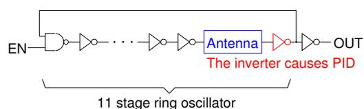
Fig. 5. 11 Stage Ring Oscillator for Measuring Frequencies
