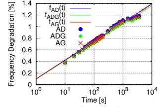
Fig. 14. BTI of AR6250 in the SOTB Process
