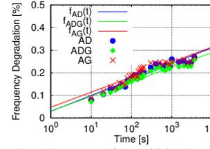
Fig. 11. BTI of AR500 in the Bulk Process
