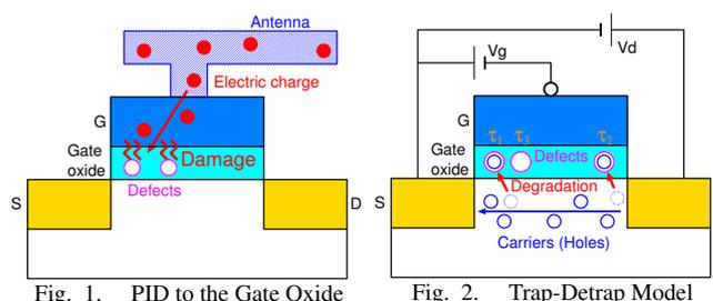
Fig. 1. PID to the Gate Oxide
