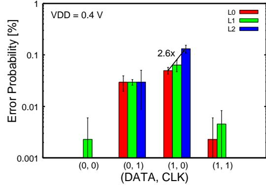
Fig. 6.  $P_{SE}$  in each condition by alpha particle irradiation. The error bars show 95% confidence.
