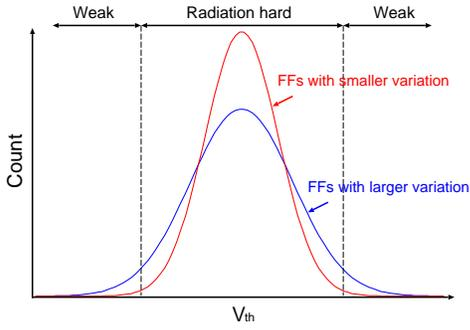
Fig. 7. Difference of radiation hardness depending on variation of MOSFETs.
