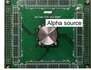
Fig. 5. Alpha test setup.
