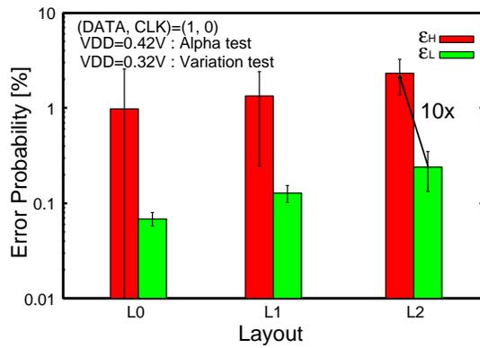
Fig. 9. Experimental results between the retention voltage and the radiation hardness of each FF. The Error bars show 95% confidence.
