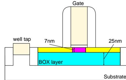
Fig. 1. Cross section of UTBB FD-SOI structure.
