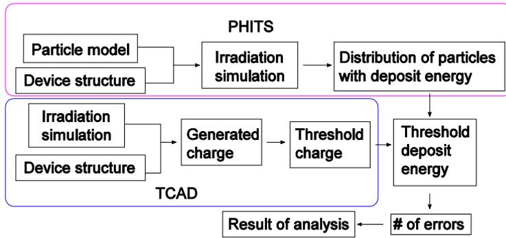
Fig. 1. Flow chart of the PHITS-TCAD simulation system.
