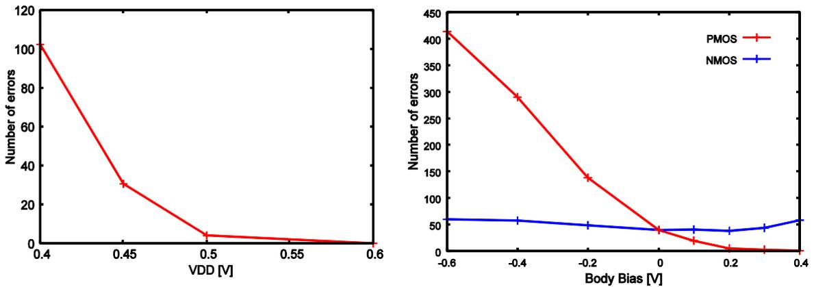
(a) The number of errors by reducing VDD according to alpha irradiation experiments.
