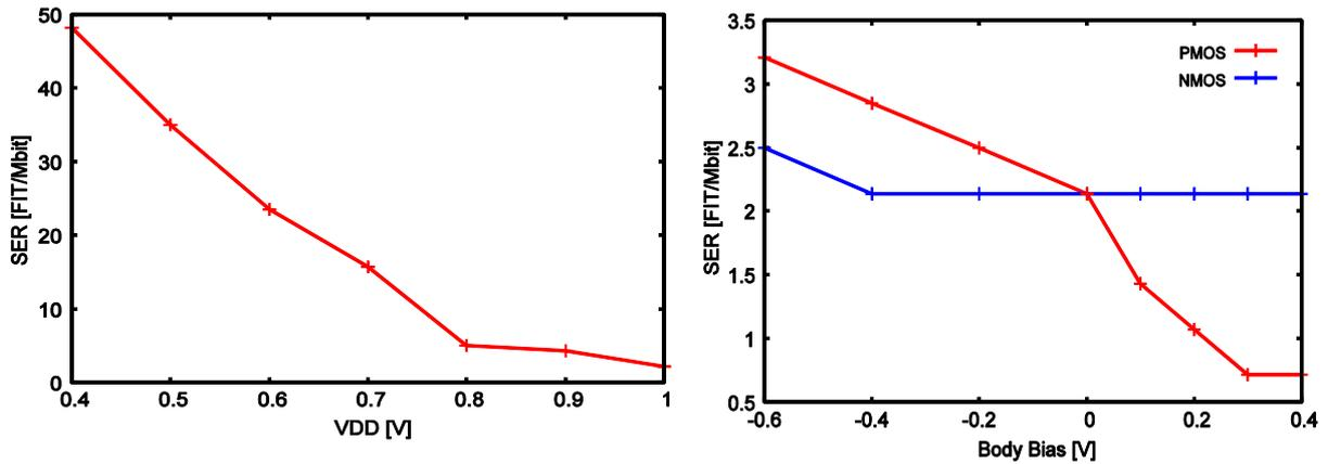
(a) The SER of reducing VDD according to simulations.
