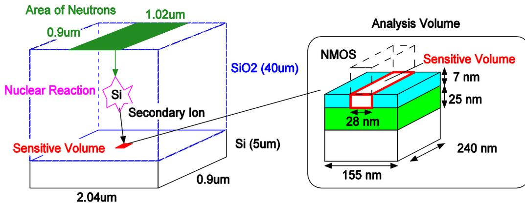
Fig. 3. Device structure used in PHITS. The sensitive volume is defined by the active area of a latch (28 nm x 240 nm) and the sensitive depth (7 nm).
