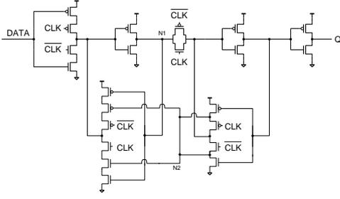
Fig. 5. Feedback recovery flip flop (FRFF)
