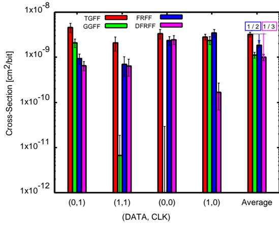
Fig. 13. Experimental results of the CSs by Kr irradiation at  $V_{dd}$  of 0.8 V.
