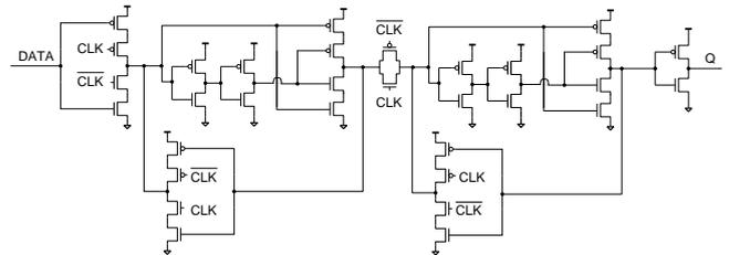
Fig. 4. Guard-gate flip flop (GGFF)
