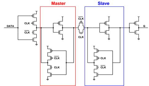
Fig. 1. Transmission-gate flip flop (TGFF)
