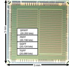
Fig. 8. Chip micrograph that contains 20,088 bit standard TGFFs, 20,124 bit GGFFs, 20,196 bit FRFFs and 20,250 bit DFRFFs.
