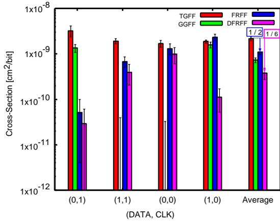
Fig. 15. Experimental results of the CSs by Kr irradiation at  $V_{dd}$  of 1.2 V.
