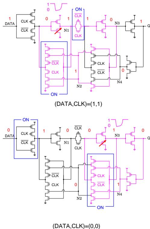
Fig. 17. NMOS transistors sensitive to a heavy-ion hit at (DATA, CLK) = (0, 0), (1, 1).
