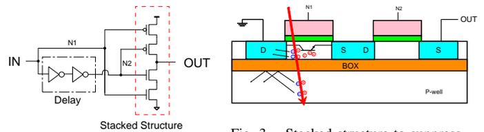
Fig. 2. Guard-gate structure
