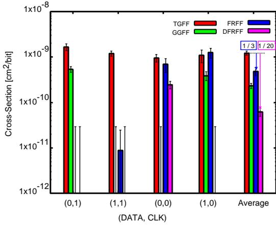
Fig. 14. Experimental results of the CSs by Ar irradiation at  $V_{dd}$  of 1.2 V.
