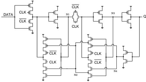
Fig. 7. Dual feedback recovery flip flop (DFRFF)
