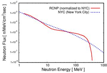
Fig. 10. Normalized energy spectrum of spallation neutron beam at RCNP and neutron at the sea level of NYC.
