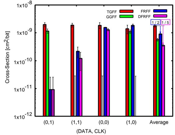
Fig. 12. Experimental results of the CSs by Ar irradiation at  $V_{dd}$  of 0.8 V.
