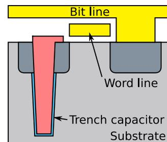
Fig. 1: Trench capacitor and planar MOSFET
