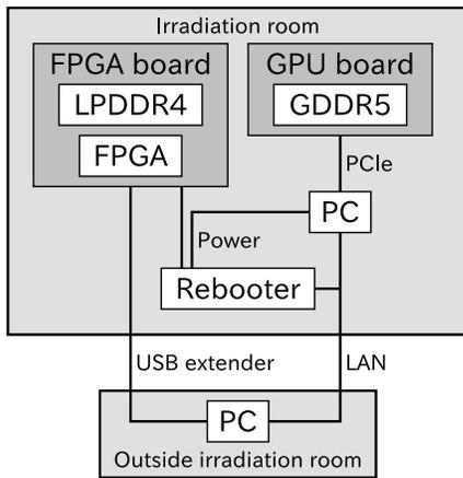
Fig. 4: Measurement system
