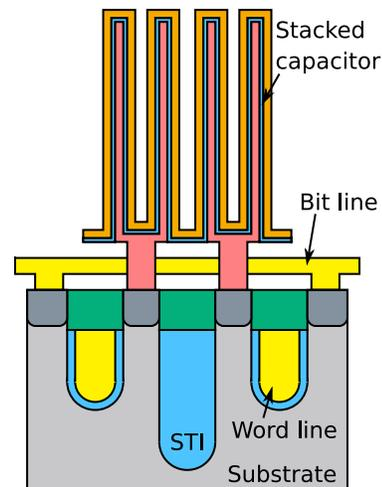
Fig. 2: Stacked capacitor and trench MOSFET
