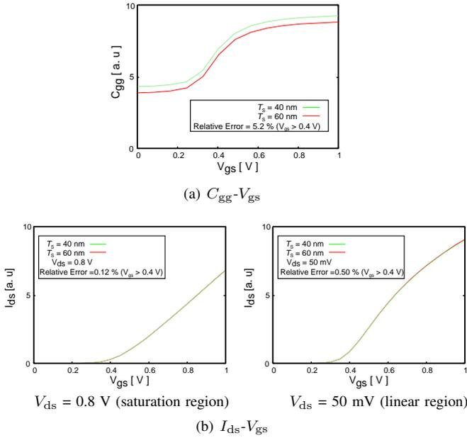
Fig. 10. Dependence of silicon thickness to transistor characteristics
