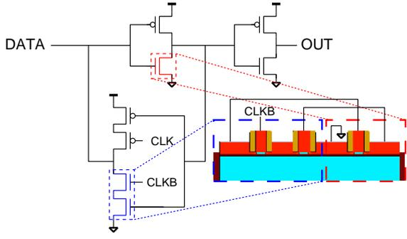
Fig. 3. Schematic diagram and the cross-sectional view of the 3D model used for device simulations.
