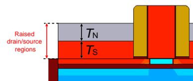
Fig. 2. Structure of the raised layer. Definition of thickness of silicon ( $T_S$ ) and thickness of nickel silicide ( $T_N$ ).
