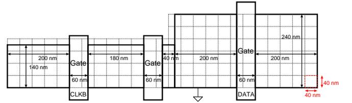
Fig. 5. Simulation setup to evaluate cross sections induced by a heavy ion with Ar and Kr. Radiation particles strike at the center of each grid.
