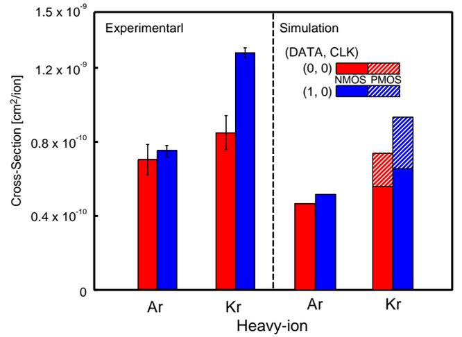
Fig. 11. Cross sections considering both of NMOS and PMOS contributions from simulations ( $T_S = 60$  nm) and experiments.
