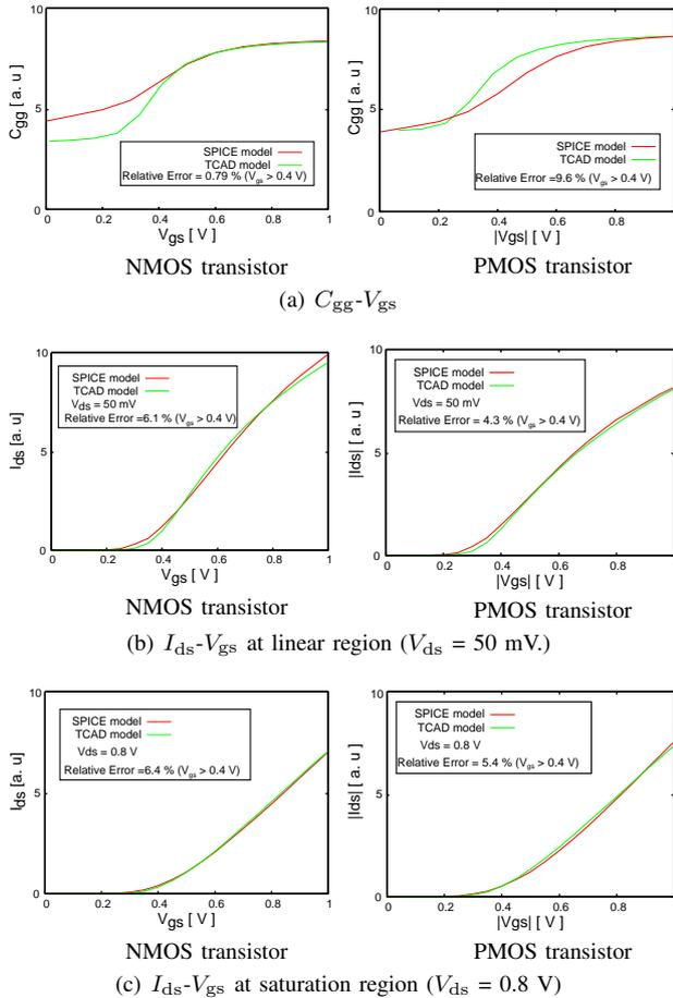
Fig. 4. (a) Simulated  $C_{gg}-V_{gs}$  characteristics at  $V_{ds} = 0$  V. (b) Simulated  $I_{ds}-V_{gs}$  characteristics at linear region. (c) Simulated  $I_{ds}-V_{gs}$  characteristics at saturation region.
