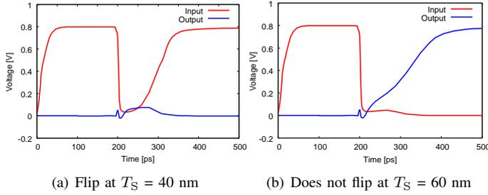
Fig. 7. DATA and OUT voltage of the tristate inverter.
