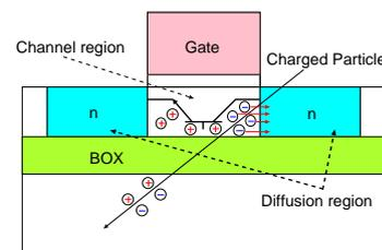
Fig. 1. Holes generated in the diffusion region are collected in the channel region and then drain-body-source parasitic bipolar transistor turns on.
