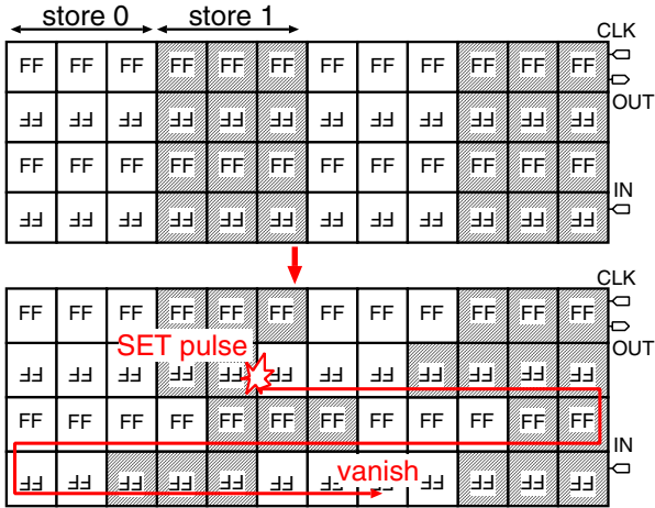
Fig. 5. Initial stripe pattern to detect an SET pulse (3bit stripe version).
