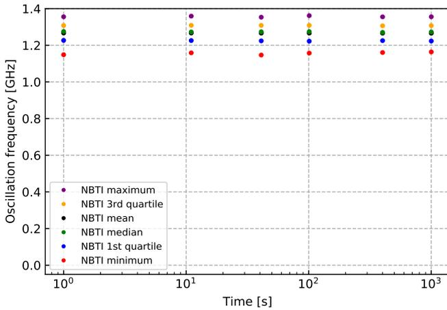
Fig. 9: Distributions of 840 NBTI-ROs at 100°C after 1 month recovery at room temperature
