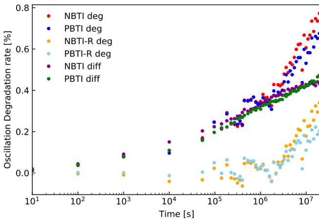
Fig. 5: Degradation rates for all ROs and difference.
