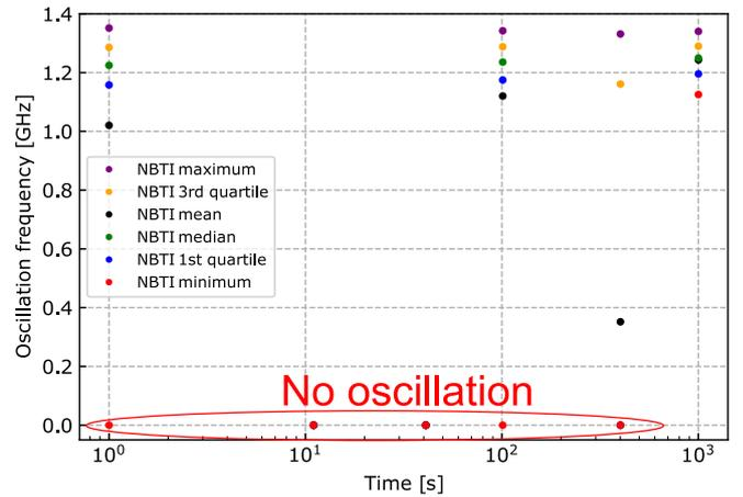
Fig. 10: Distributions of 840 NBTI-ROs at 120°C after 1 month recovery at room temperature
