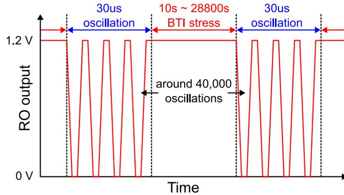
Fig. 4: Measurement method of BTI-induced degradation indicated by RO output
