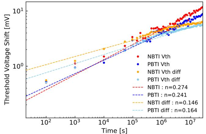
Fig. 6: Threshold voltage shifts and fitting results.
