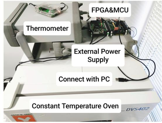
Fig. 2: Photograph of long term measurement system [4].
