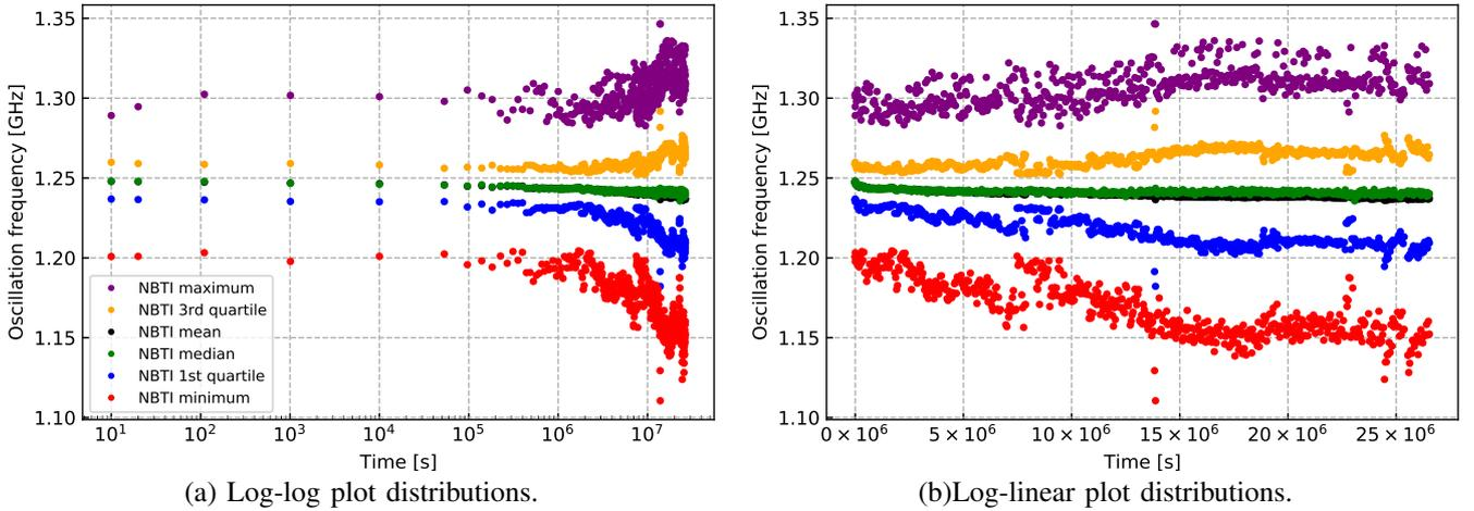
Fig. 8: Distributions of 840 NBTI-ROs in long-term measurement.
