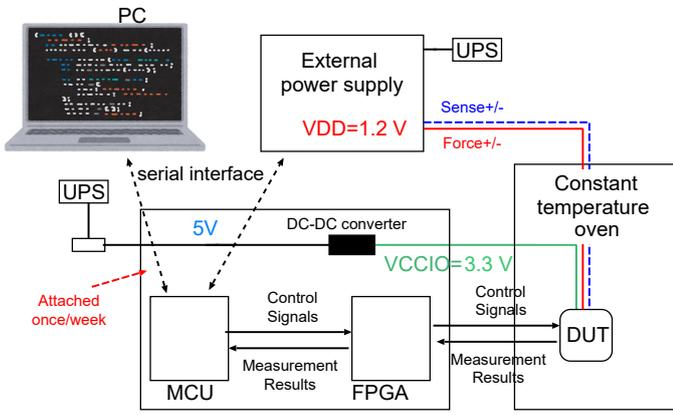
Fig. 1: Long term measurement system [4].
