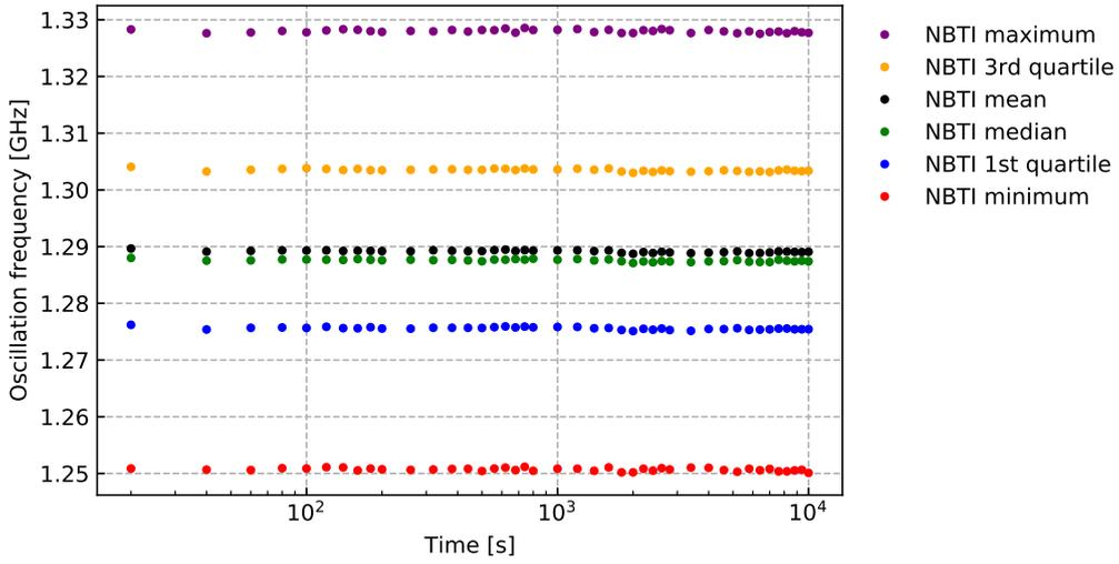
Fig. 7: Distributions of 840 NBTI-ROs in short-term measurement
