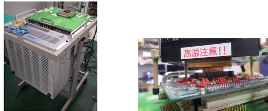
Fig. 1: Short-term measurement system of aging degradation using an engineering tester (left) and a Peltier element (right).
