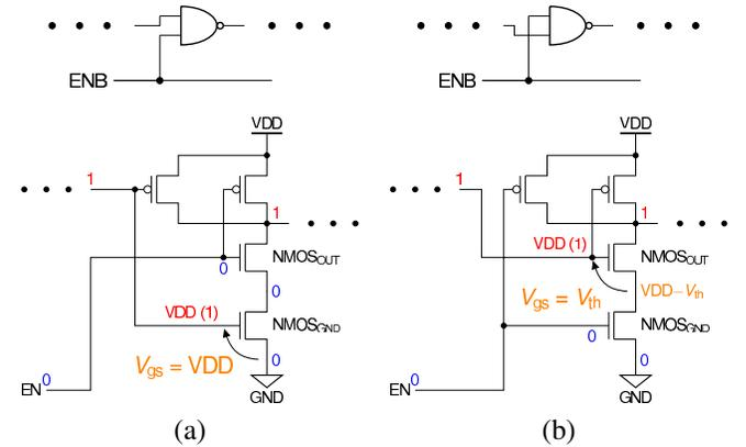
Fig. 6. NAND RO in transistor level. (a) PBTI-sensitive RO. (b) PBTI-insensitive RO.
