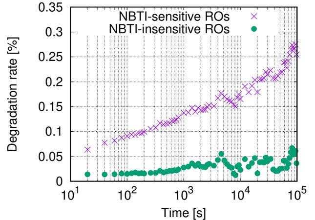
Fig. 11. Measurement results of NBTI-induced degradation.
