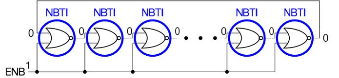
Fig. 5. RO composed NOR gates. NBTI becomes dominant when RO stops.
