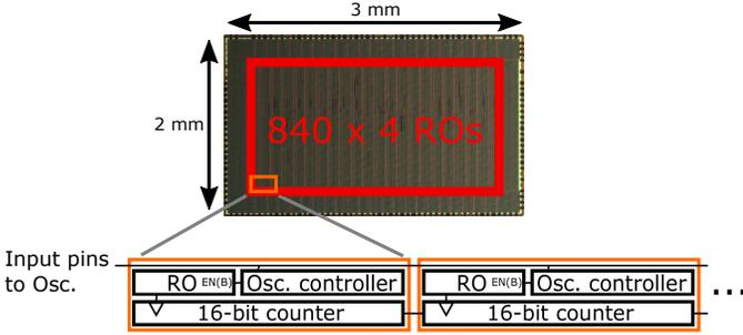
Fig. 8. Test chip micrograph. The number of oscillations is counted by embedded 16-bit counter.
