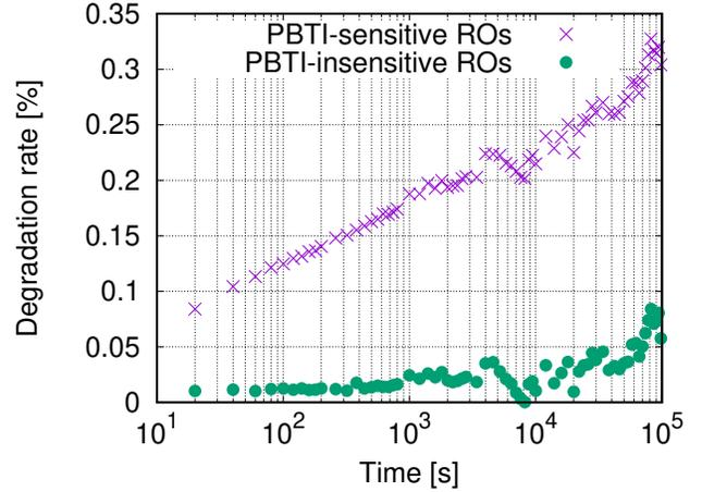
Fig. 10. Measurement results of PBTI-induced degradation.
