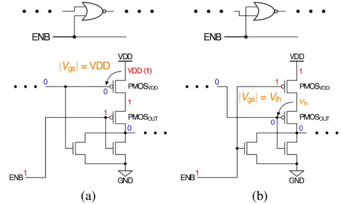
Fig. 7. NOR RO in transistor level. (a) NBTI-sensitive RO. (b) NBTI-insensitive RO.
