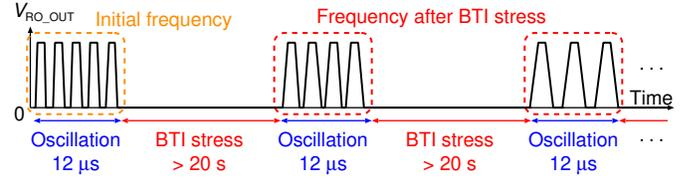
Fig. 9. Measurement flow of BTI-induced degradations.
