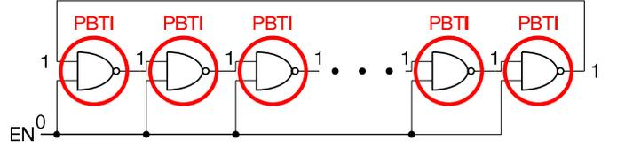
Fig. 4. RO composed NAND gates. PBTI becomes dominant when RO stops.
